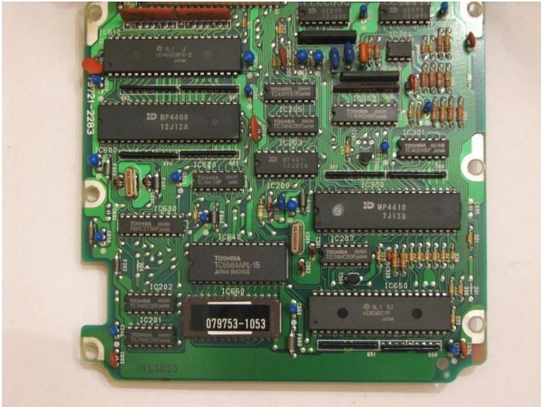
We need to remove IC660 (the chip with the stick on label at the bottom left of the above picture, closeup pic below). The board will also be silk screened with IC660.
