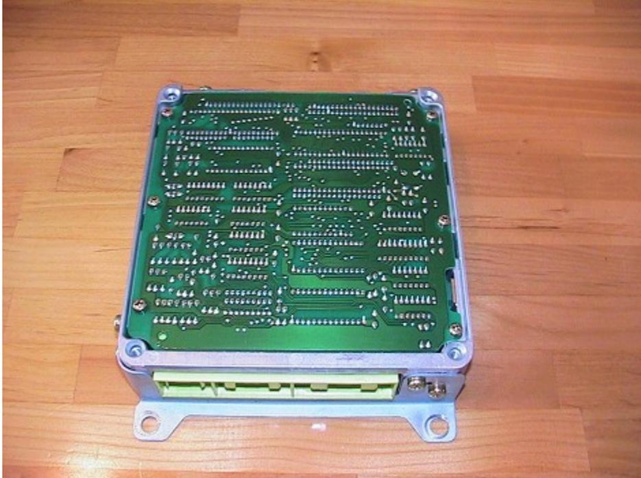
This is the backside of the digital board and where we'll be making our changes. Remove the 6 phillips screws around the edge and gently fold out the board.
