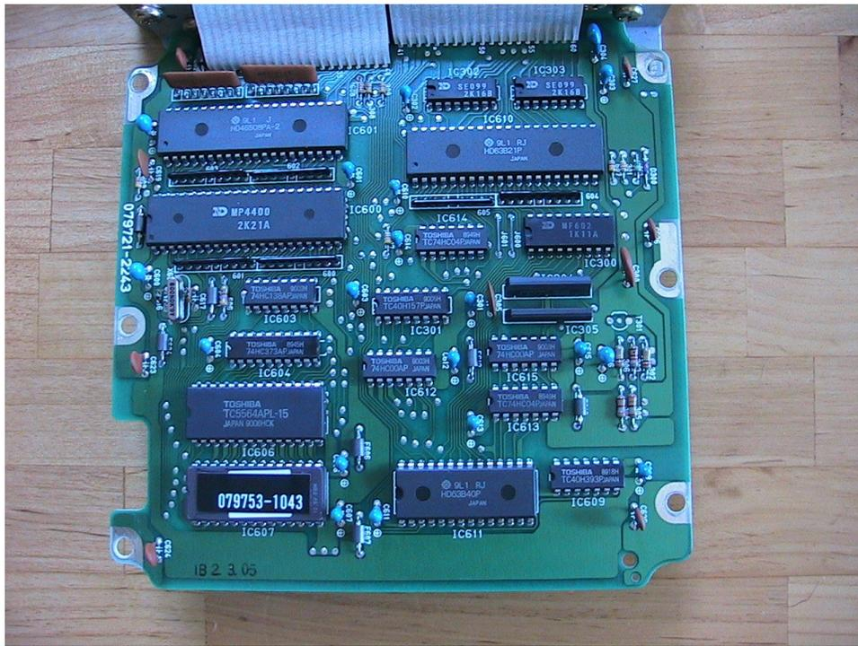
We need to remove IC607 (the chip with the stick on label at the bottom left of the above picture, closeup pic below). The board will also be silk screened with IC607.
